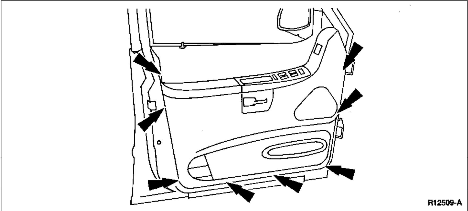
5. Start in a lower corner and work around the panel and separate the front door trim panel (23942) from the front door (20124) to disengage the pin-type retainers.
